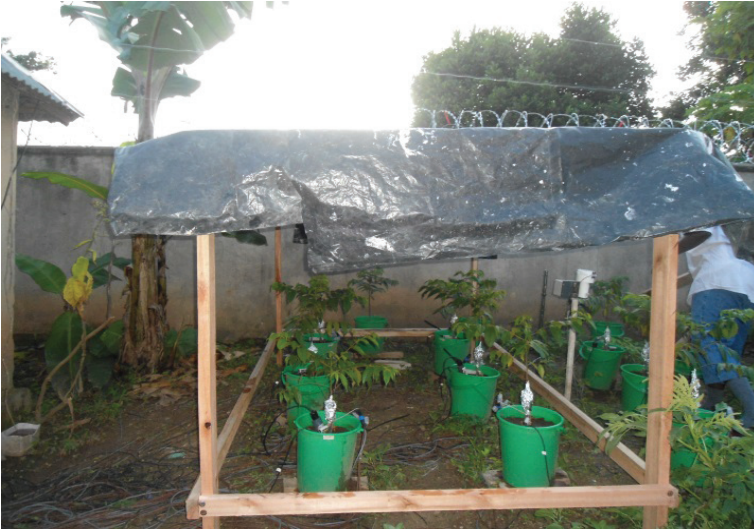
Figure 2.2 Set up at study site showing from extreme left, the drought followed by watered and on the extreme right, the rain-fed. The black plastic sheeting is the cover anchored down during rainy days and during the night
