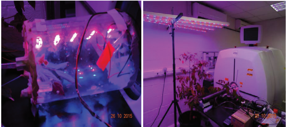
Figure 3.2 Left to right: An excised M. eminii branch with secondary branch placed in chamber and inserted into a radiation shield chamber
