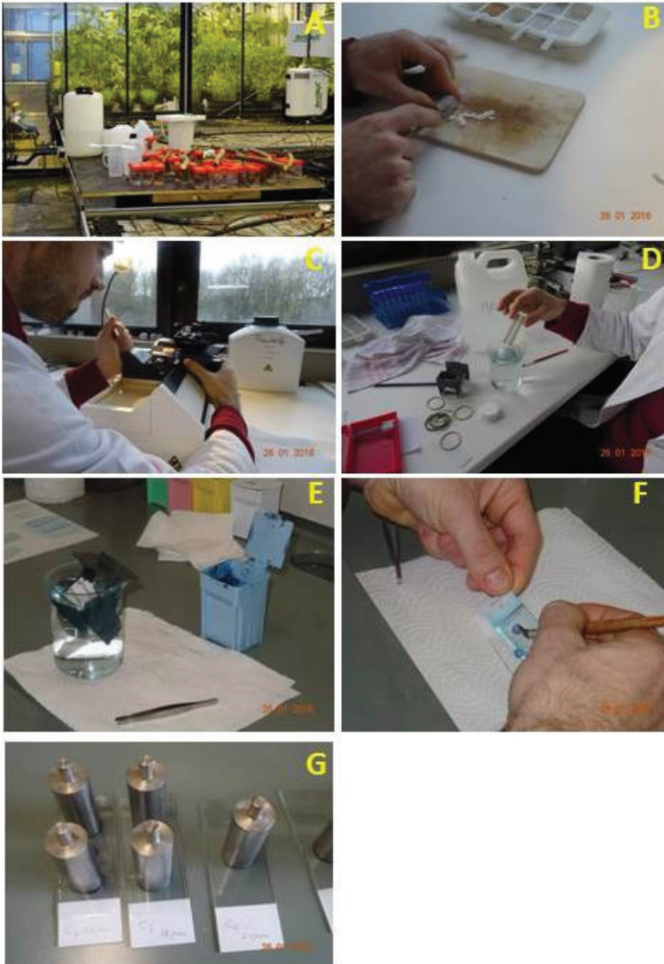
Figure 4.4 Illustratively from top to bottom and from left to right: the storing of the wood samples in the concoction as described in the text at the tropical greenhouse at ILVO (A). The reshaping of the mummified branch (B) and making of thin sections (C). The thin sections secured with a rubber band between nylon and glass slide were dipped in water to rinse off excess PEG (D). These were then dipped in alcohol of varying concentrations in the trash bin-like containers (E). Excess alcohol was drained by tilting the slides, Euparal added and setup covered using microscope cover glasses (F). Weights were placed on them and allowed to dry (G).
